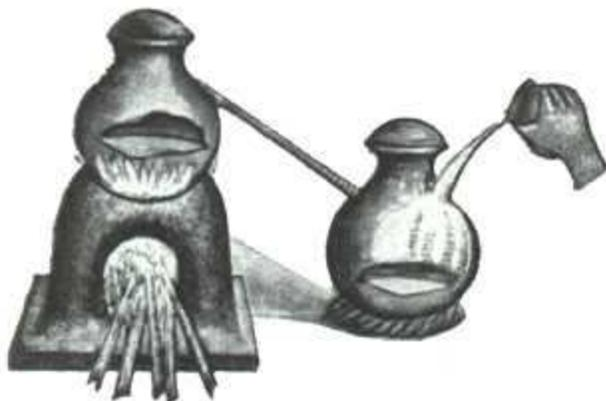
Distillation apparatus using simple hand cooling for the receiver.
