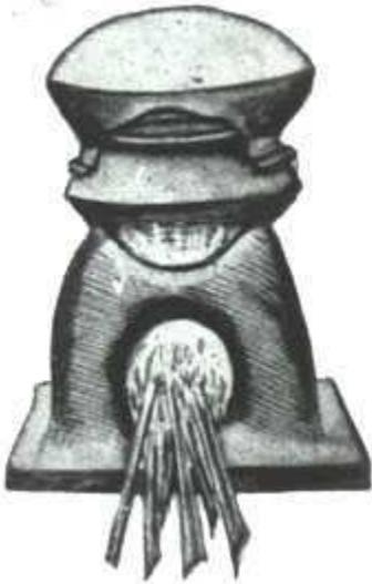
Sublimation apparatus. The larger upper vessel is cooled by air.
