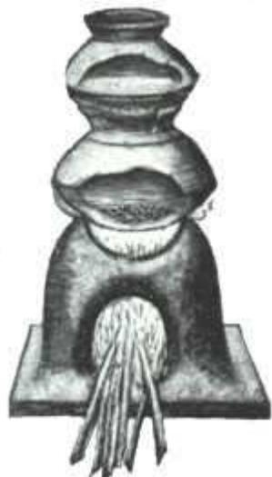
Sublimation apparatus. The upper dish is filled with cold water.
